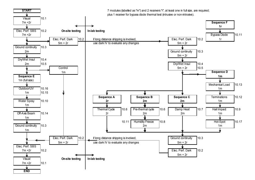
IEC62108 – CPV Modules and Assemblies: Design Qualification and Type Approval
