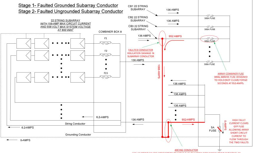
HIGH CURRENT CAUSES CONNECTION TO MOVE SLIGHTLY FROM GROUNDING POINT INITIATING AN ARC THAT CONTINUES UNTIL ARRAY COMBINER FUSE CLEARS IN 60 SECONDS
