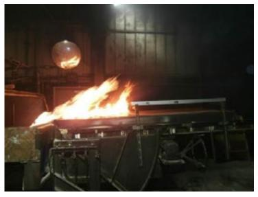
*Figure 5.* Example experiment illustrating first to ignite, second to ignite concept with 48-inch offset (low slope roof with low slope FR EPDM, noncombustible PV surrogate, five-inch gap)
