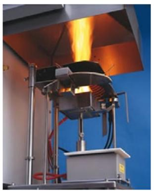
Figure 4. Cone calorimeter test apparatus (ASTM 1354).
