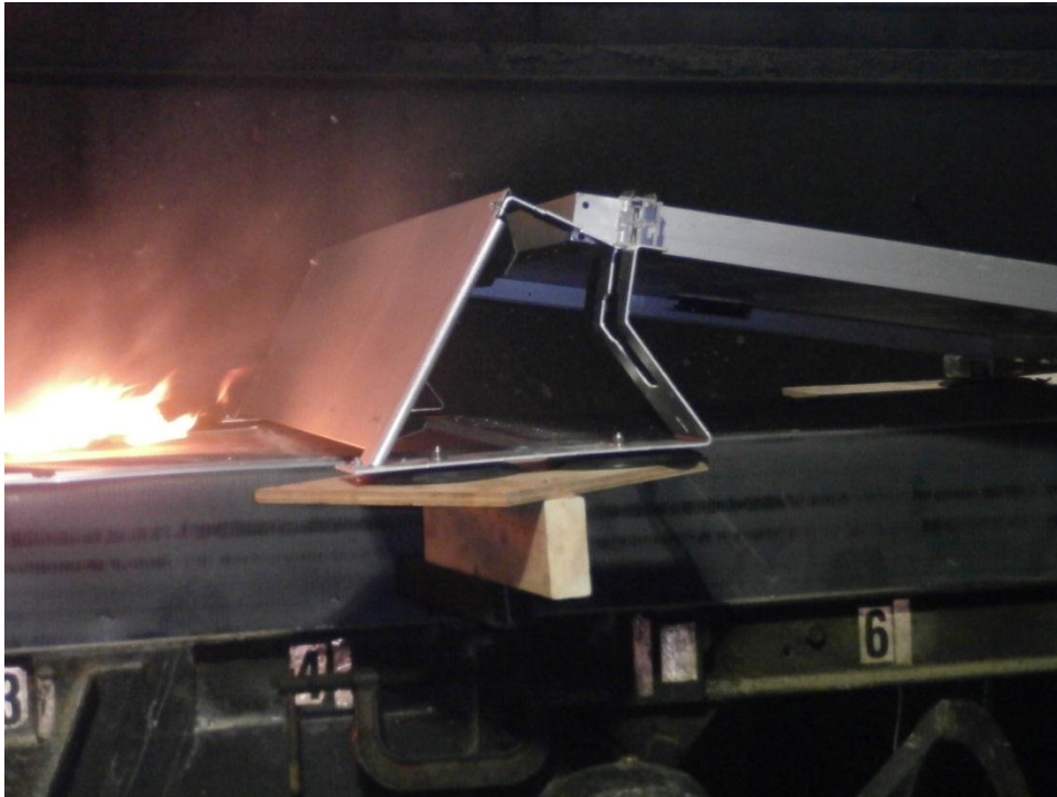
Figure 3 – Figure Illustrating Spread of flame of North Exposure PV / FR EPDM System – “Pedestal” mounting.
