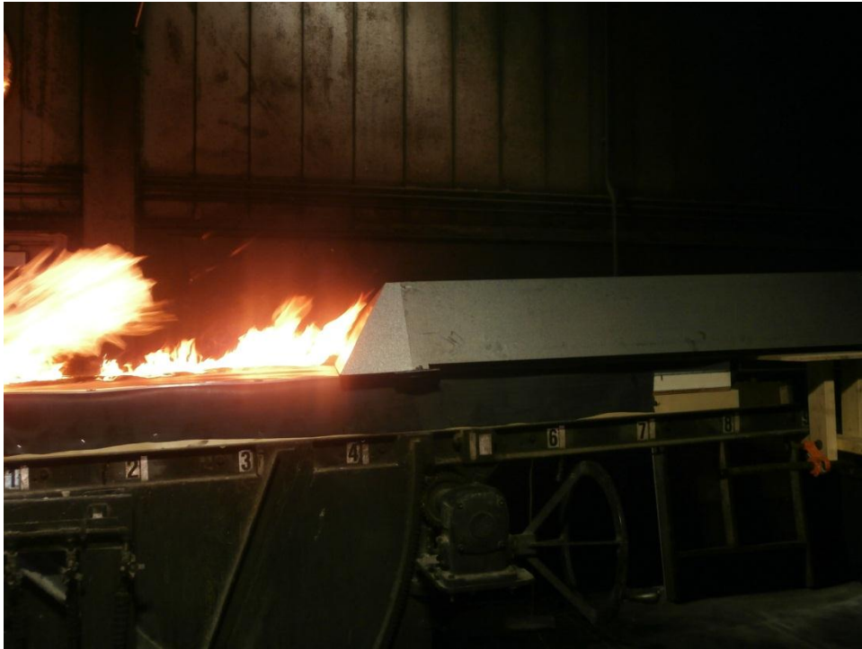
Figure 5 – Figure Illustrating Spread of flame of East/West PV / FR EPDM System – “Pedestal” mounting.
