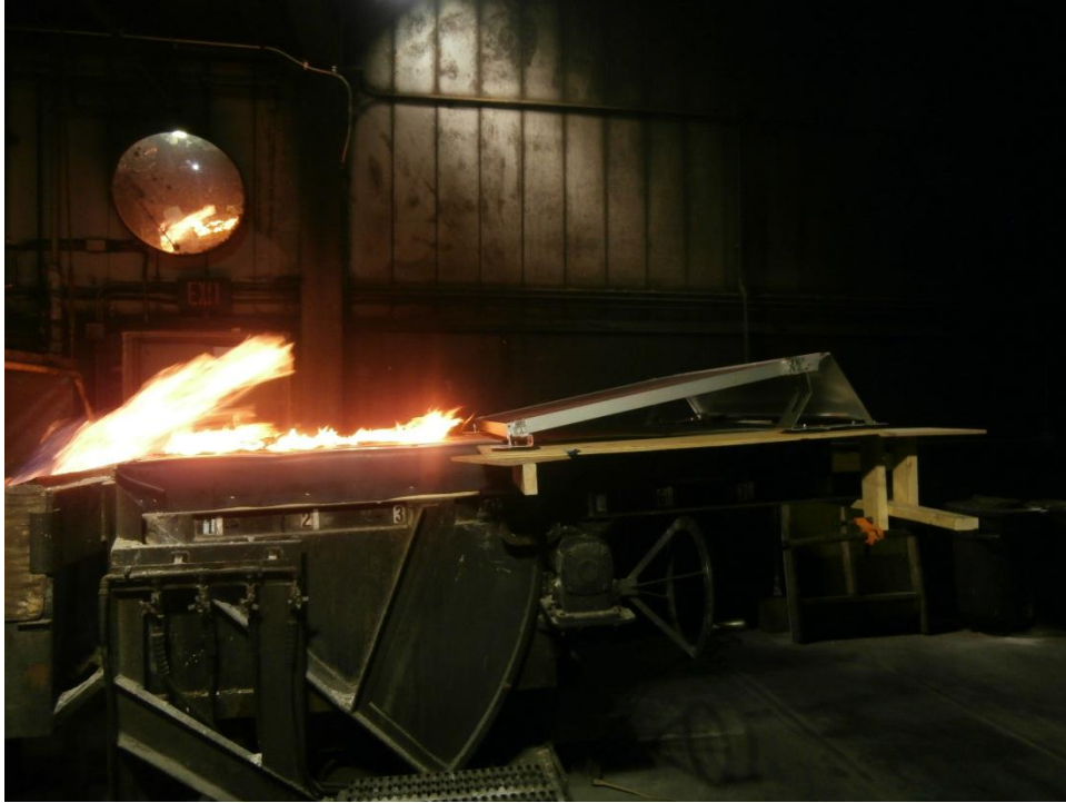
Figure 7 – Figure Illustrating Spread of Flame of South Exposure PV / FR EPDM System – “Platform” mounting.
