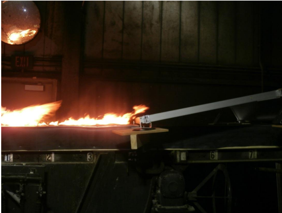
Figure 2 – Figure Illustrating Spread of flame of South Exposure PV / FR EPDM System – “Pedestal” mounting.
