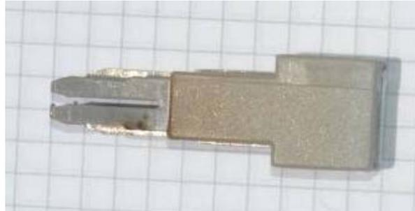
**Bridge connectors with damaged (slightly burned) contacts that were used to join the two halves of the PV array in the middle of the array connector box. In this case, due to the low voltage available to sustain the arc (about  $0.2 V_{MPP}$ ), no arc occurred.**
