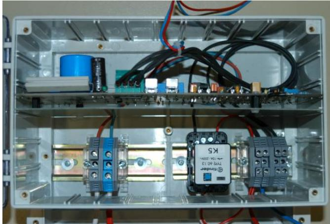
The arc detector (AD) with IDU which was used for these tests performed in autumn 2006 was composed of parts that were still available from earlier projects. Many parts were used that would not be needed for an AD integrated into an inverter.
