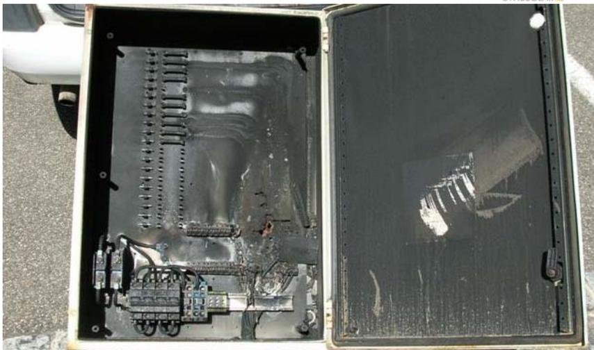
**After opening, additional oxygen could enter the cabinet and a catastrophic fire occurred that destroyed the cabinet completely.**
