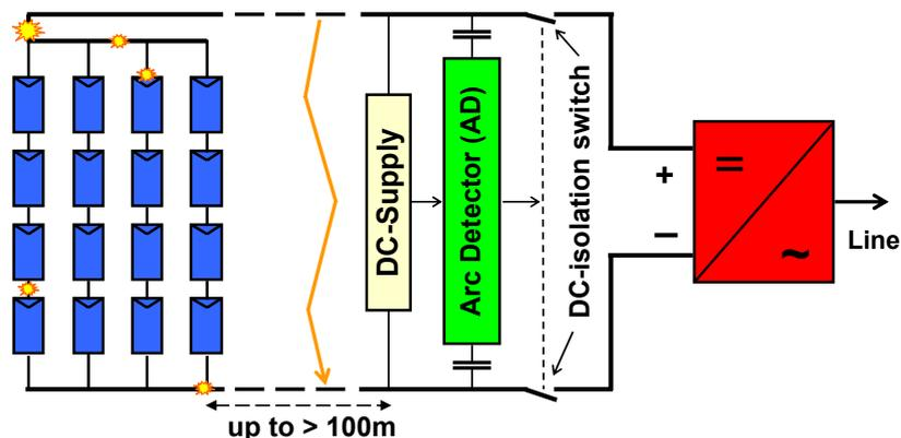
When an electrical arc occurs on the DC side, in a *combination of two resonant circuits* a high-frequency signal is detected. After certain checks the isolation switch is activated and the DC side of the inverter is disconnected.
