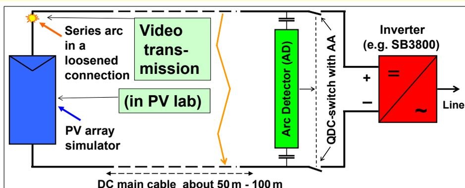
Upon recognition of a series arc in the loosened connection, the arc is interrupted by means of an electromechanical QDC switch.
