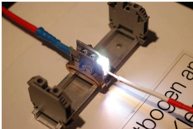
With a loosened connection an arc occurs, which is recognised by the AD and switched off immediately.
