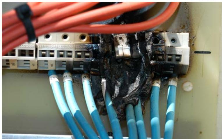
Close-up view of the origin of the fire. A soldering point on the PC board or a connection gradually warmed up and finally melted, developing an electrical arc causing the fire ( $V_{MPP}$  was about 500V).
