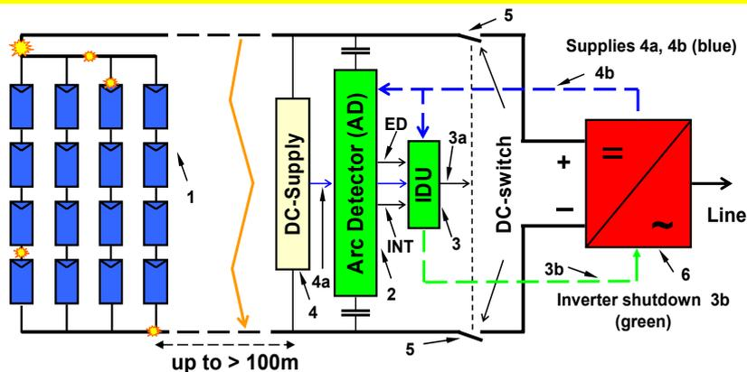
**Block diagram of an improved AD for a reliable remote detection and interruption of dangerous arcs on the DC side of PV plants.**
