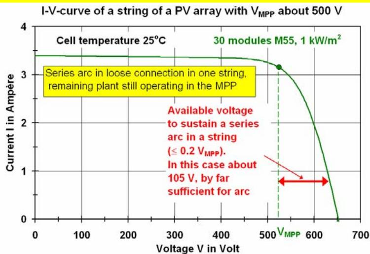
**A high MPP-voltages  $V_{MPP}$ , series arcs are possible**
