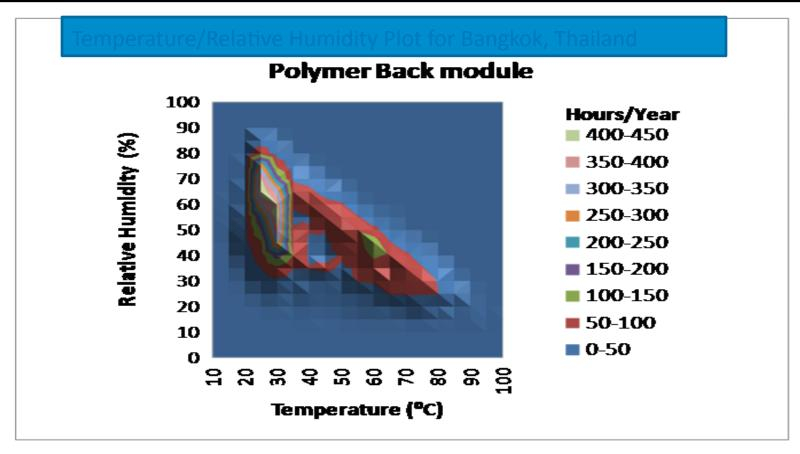
Modeling of humidity levels in back of PV module with polymeric backsheet in Bangkok, Thailand.
