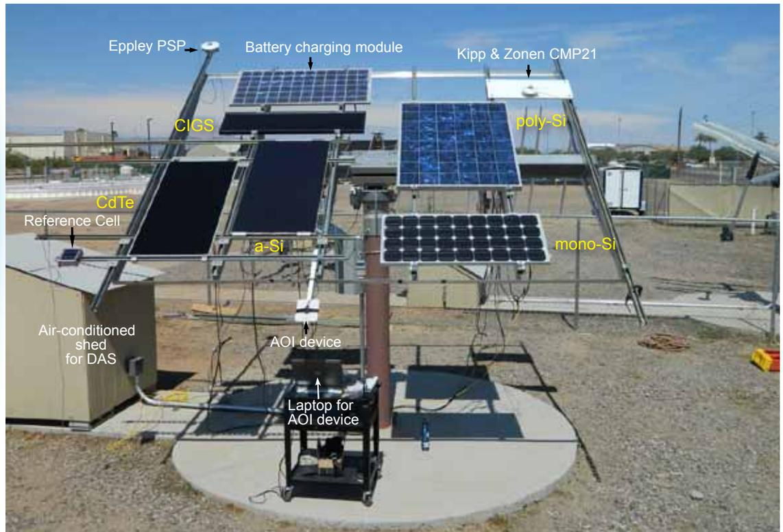
Figure 4. AOI measurement setup on a two-axis tracker.
