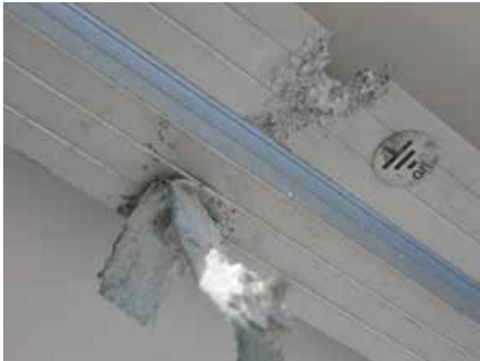
*Figure 1:* Corrosion between copper ground braid, stainless steel screw, and aluminum frame.
